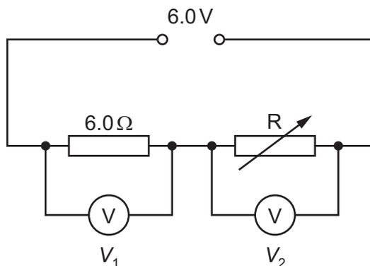
When R is adjusted to 6.0 Ω, the voltmeter readings  $V_1$  and  $V_2$  are equal.
